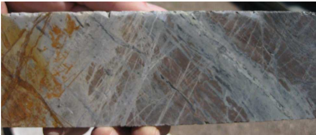
Multi-stage silica veinlets/flooding with pyrite stringers in core below the Mirador pit
