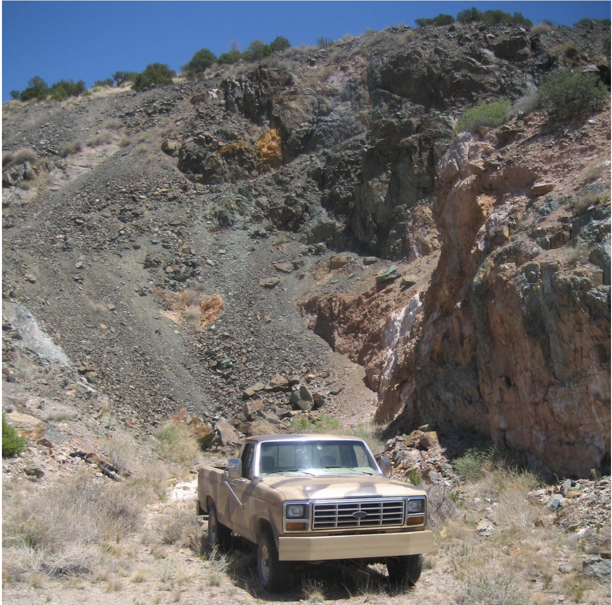
Milagros open cut: Remnants of the gold-silver, vuggy quartz-iron oxide vein are exposed on the high wall and in the left-center of the photo.
