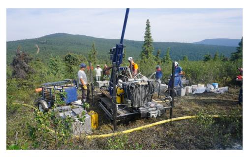
This company is revolutionizing prospecting and exploration in the Yukon by employing low-impact, easily maneuverable drill equipment to test targets quickly and at a much lower cost with less ground disturbance and no permitting requirements versus standard core drilling:
