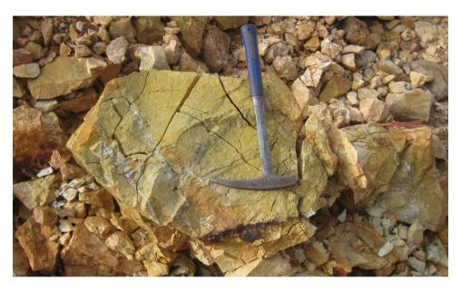
Fine-grained silica replacement of rhombohedral calcite crystals, typical of high-level epithermal vein deposits:
